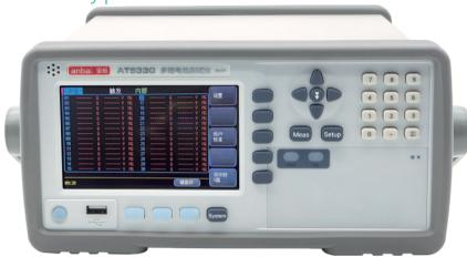
The AT5330 multi-channel battery tester is a micro desktop instrument that uses a high-performance 32-bit ARM microprocessor to control fully automatic real-time detection. It can scan and test the internal resistance and voltage of 30 channel batteries. The instrument can test a resistance of 0.001m  $\Omega$ ~3k  $\Omega$ , a DC voltage of 0.0001V~60.000V, a maximum resistance of 30000 display
