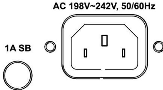
To prevent electric shock, be sure to turn off the power switch and unplug the AC power cord before checking or replacing the fuse.
