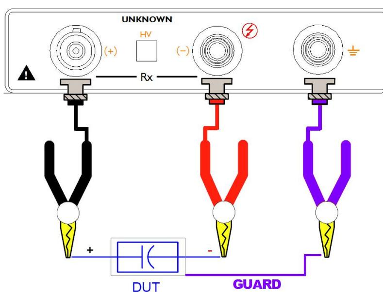
Note: If your device under test has a shielded enclosure, it cannot be connected to the positive and negative poles.
