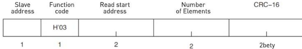
The function codes of the read-out registers are 0x03.
