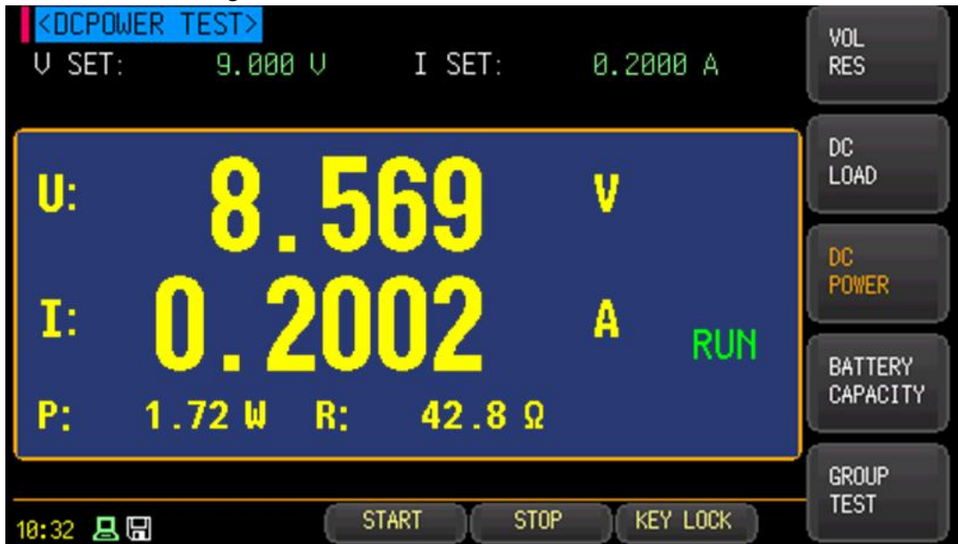
Picture 4- 6 < DC Power Test > Page
