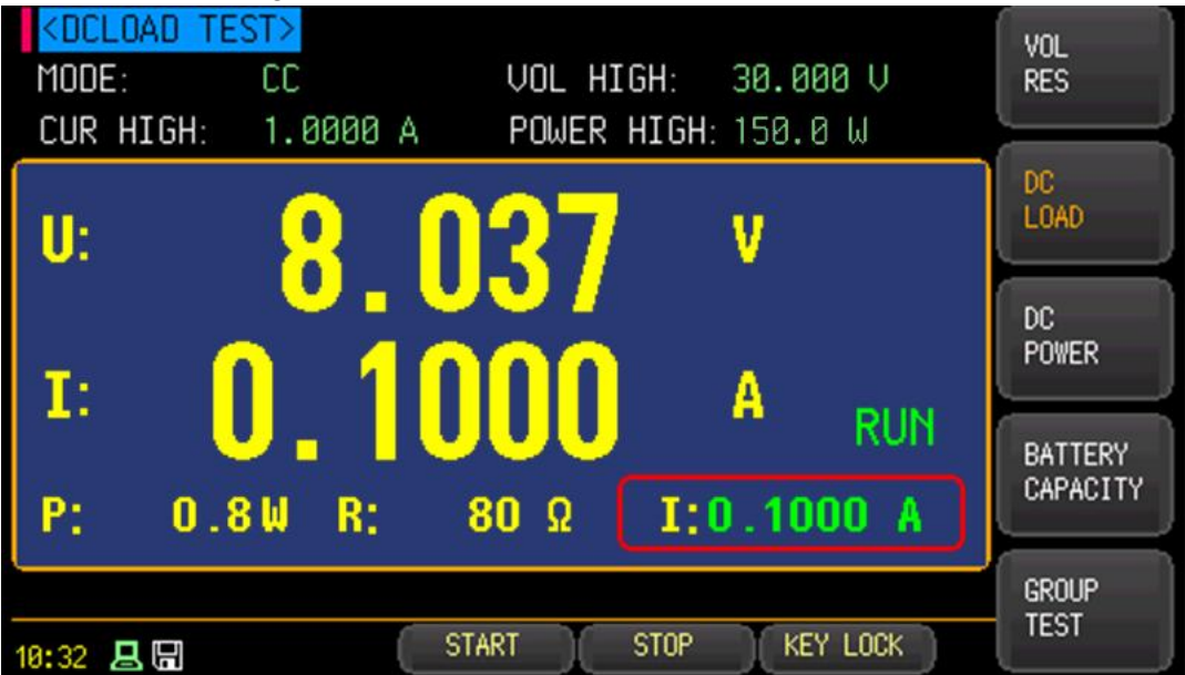
Picture 4-5 < DC Load Test > Page
